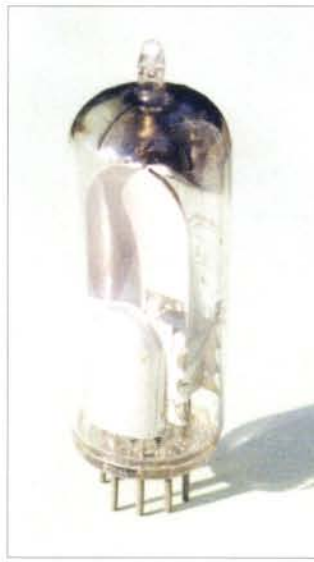
Fig. 1: The EM81 'Magic Eye' indicator valve. Note that this valve uses an internal metal fluorescent screen (see text).
