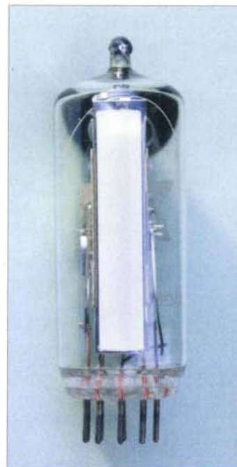
Fig. 6: Mullard's EM87, employing an 'on glass' fluorescent screen, was specifically designed for use in tape recorders (see text).
