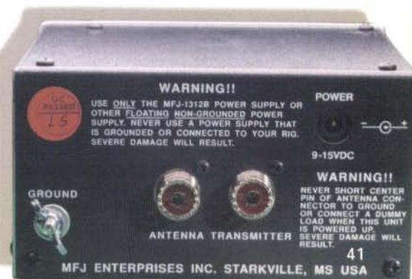
Fig. 4: The rear panel of the remote control unit, with important and appropriate warnings regarding the power supply (see text).
